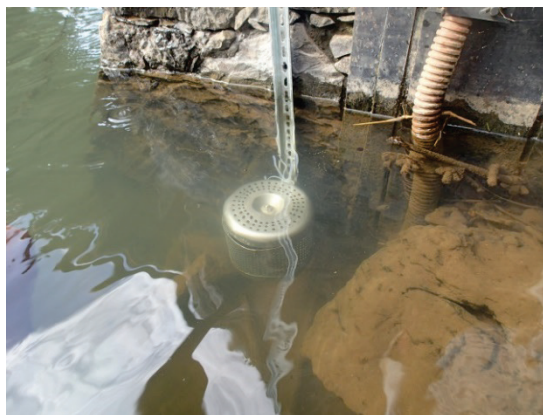
Figure 4. Cage POCIS immergée station Grand Galion
