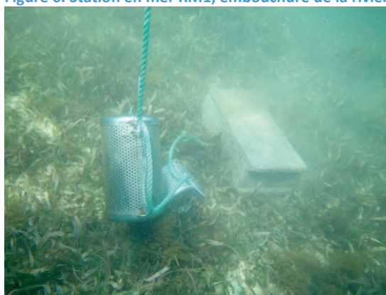
Figure 8. Cage POCIS immergée, station RM3.
